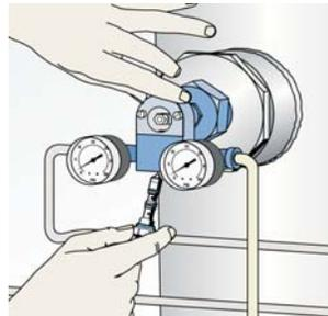
Turn on supply pressure to the controller. Adjust the MIZER® Pilot Valve in and out until the desired pressure is achieved
